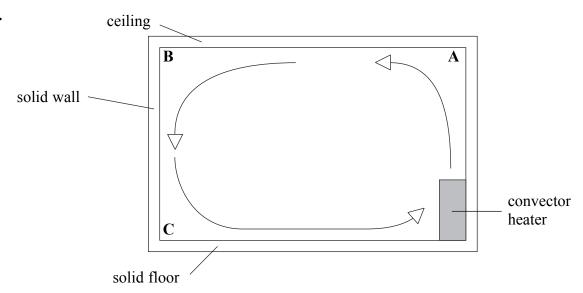
(a) The room shown is heated by a convector heater. The arrows show the direction of movement of the air within the room.Is the highest temperature at A or B or C?
